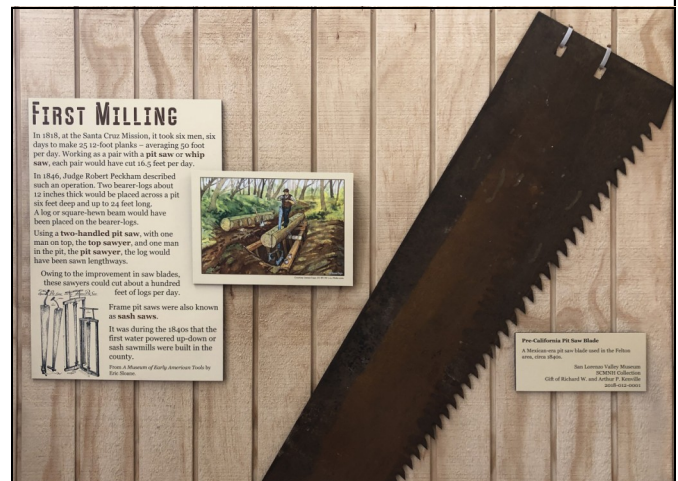
Mexican-Era Pit Saw Blade Used in the Felton Area circa 1840. SCMNH Collection, 2018-012-0001.
